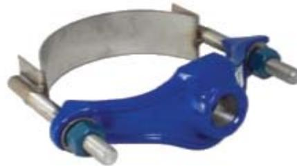
*Note: Select desired saddle O.D. range which specifically matches outside diameter of pipe. Saddles for C-900 shall be sized to the exact O.D. size for proper fit. Single Strap Saddle is approved for new 1-inch water services only which are installed on dry water main, sized 4-inch through 10-inch.*
