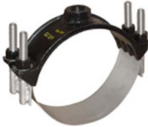
*Note: Select desired saddle O.D. range which specifically matches outside diameter of pipe. Saddles for C-900 shall be sized to the exact O.D. size for proper fit. A double strap saddle will be required for all wet taps and are acceptable for installation on dry water supply mains (all sizes).*
